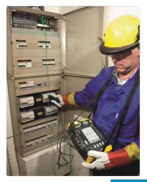
In domestic, tertiary or industrial environments, these new multi-function installation testers can be used to check an electrical installation's compliance with the applicable standards. This verification is mandatory to ensure that the installation is not hazardous, whatever the type of building tested (domestic, public building, industry, etc.).
