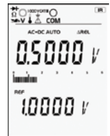
ΔREL Mode Displays relative values with respect to referenced measured value
