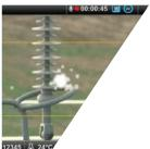
HD corona camera with features that boost corona detection and visualization. LuminarHD is the optimal choice when asking to streamline monitoring tasks. Outstanding optics and sensitivity to UV ensure unparalleled performance and clear display of pinpointed corona from far away and nearby. High definition recording lets users see more when analyzing the recorded media.
