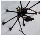
micROM<sup>HD</sup> is a state-of-the-art HD corona camera for UAS that sends in real time footage and data to maintenance teams. micROM<sup>HD</sup> provides both visual and UV video and images. Seeing corona is important to find voltage related faults and identify problems that cannot be seen with thermal imaging. The acquired data is used to fix, assess risks and troubleshoot systems. micROM<sup>HD</sup> is a perfect match for UAS, making UV imaging from air easier than ever.
