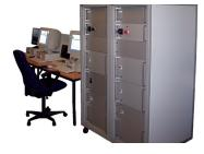
A test system designed for Circuit breaker manufacturer can be fully or partially automatic. The same software BTS11 is used as in our field testers SA5 and SA10, this makes it easy to compare
