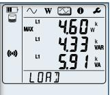
Max aggregated values of measurements and energy.
