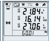
Real-time updates are displayed for voltage (V), current A) active power (P), reactive power (Q), apparent power (S), frequency (Hz), power factor (PF).
