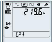
Active energy (Wh), reactive energy (varh), apparent energy (VAh). The energies displayed are the total energies, of the source or of the load. (The "h" symbol is not displayed on the screen. You will see W, VA, var for Wh, VAh and varh. Downloaded recordings will show the "h")
