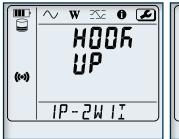
Hook up, Wi-Fi, aggregation period, can be configured from the front panel of the PEL 52. Current ratios and number of turns need to be configured via the PEL
