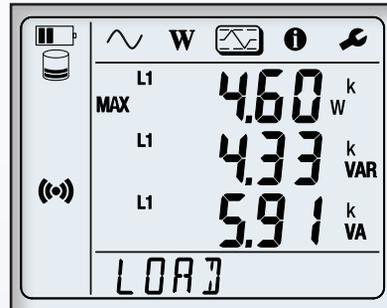
Max aggregated values of measurements and energy.
