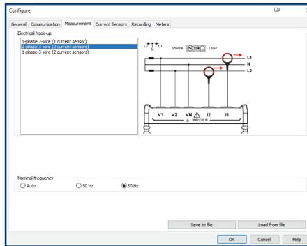
The Measurement tab specifies the electrical distribution system, voltage ratios, nominal frequency and current probe options and ratios.
