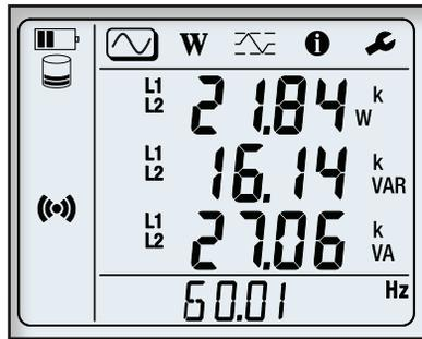
Real-time updates are displayed for voltage (V), current (I) active power (P), reactive power (Q), apparent power (S), frequency (Hz), power factor (PF) and phase shift ( $\phi$ ).
