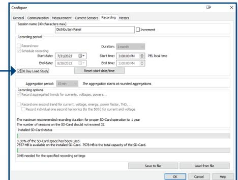
Configure the PEL to measure and record over a user selectable recording period. Select demand intervals and view available memory for data storage on the Recording tab.
