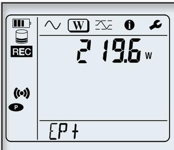
Active energy (Wh), reactive energy (varh), apparent energy (VAh). The energies displayed are the total energies, of the source or of the load.
