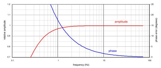
A good low-frequency response is useful when monitoring power-frequency transients where the wave-form can have a 'DC offset' which lasts for a few cycles.
