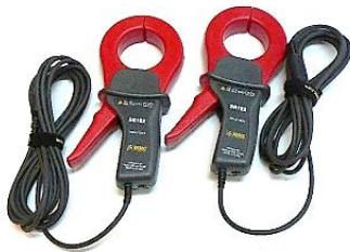
Selective/Stakeless Current Clamps 2x SR182 with 4m leads Items # 2135.72
