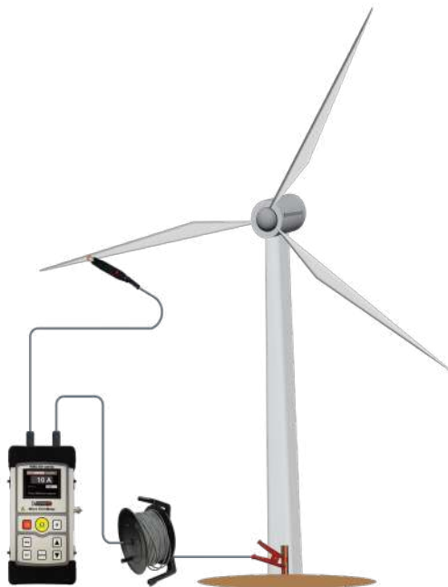
Wind turbines – lightning protection systems testing using RMO-EH Series
