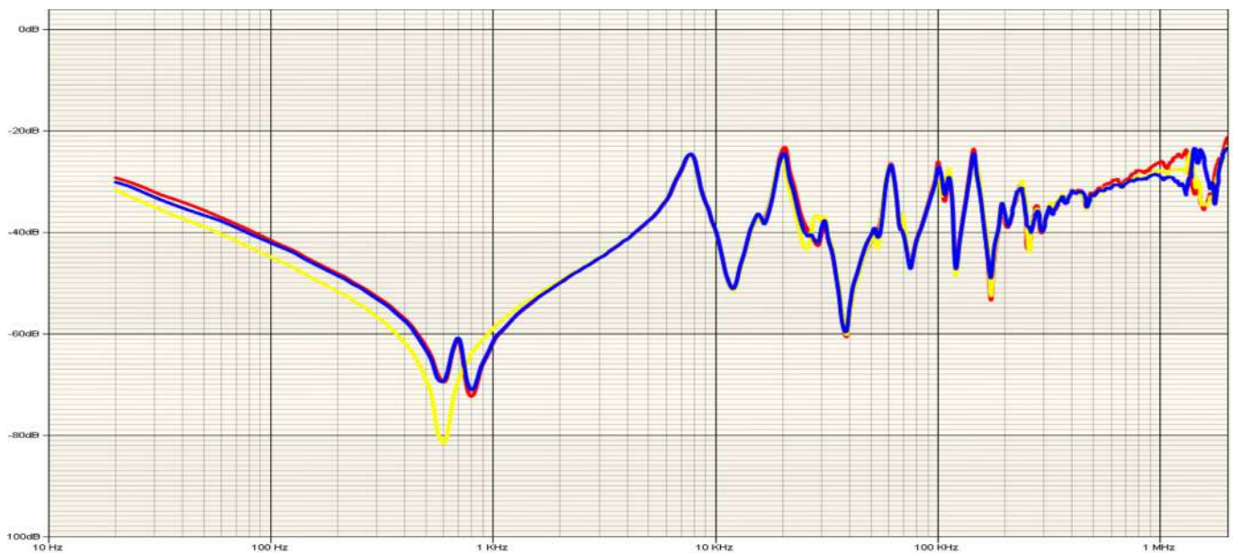
Sweep frequency response analysis trace
